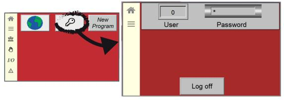
There are three different user levels on user interface. First level is for operator, levels two and three are for supervisor and level four for T-Drill service.
