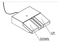
The track operating pedal is marked with stickers, which is the up, and which is the down movement of the roller track. A hand control is also available.
