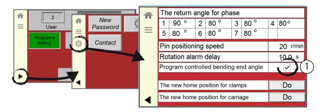
USER2 screen, tap "gear"-button and tap to check and activate "Program controlled bending end angle" function in flanging program: Set bending end angle when making the program. (Without setting, the bending end angle is 90°)
