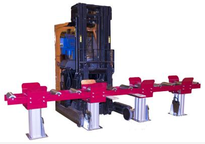
Use a forklift truck to move the roller track. Be careful with the balance, do not let the track tip over.
