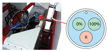
All angle adjustment plates have to be removed before starting to make settings of the angle sensor (Angular Position Transducer). The setting is not accurate with adjustment plates!
