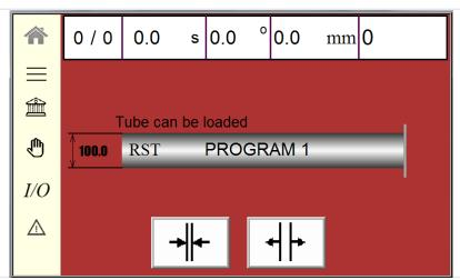
Next runs of the program: The machine will only inform above program name: "Tube can be loaded".
