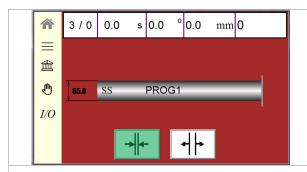
Adjust tube diameter and flange length. Load the correct flanging program to the machine.
