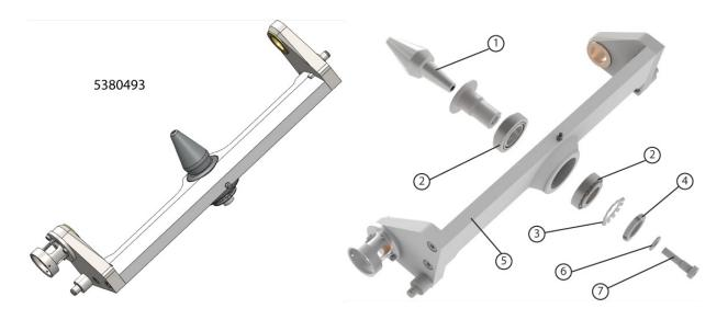
Swinging arm assembly 5380493: 1. Forming pin, 2. Bearing, 3. Spring washer, 4. Lock nut, 5. Swinging arm, 6. Washer, 7. Fastening screw of the pin (M10 socket head cap screw, 8mm key)
