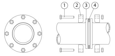
Flanged joint: 1. Bolt, 2. Loose flange, 3. Tube, 4. Sealing
