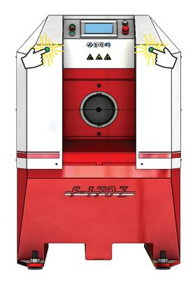
Push both two-hand control buttons simultaneously to run the clamps to READY position.
