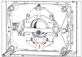
1. Angle plates on the machine body. Each fixed with 2 M5x16 socket head cap screws (3mm tool).
