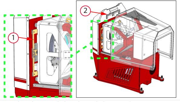
1. Backstop plate, 2. Extra backstop plates on the depository rack.
