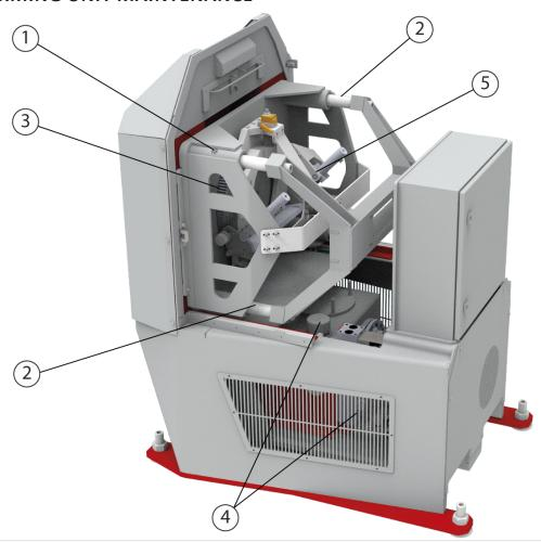
1. & 2. Flanging unit bearings and slides, 3. Rotation motor gear wheels, 4. Hydraulic system and hoses, 5. Flanging unit maintenance
