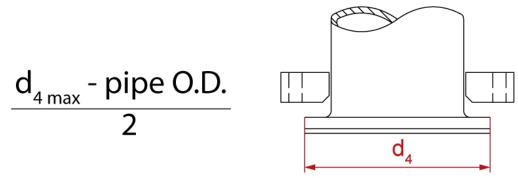
Tube material has great influence to the flange forming. Also the pipe can be either oversize or undersize. That is why it is highly recommended to test the adjustments to a scrap pipe.
