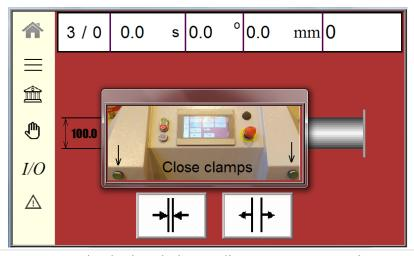
If the clamp is not completely closed, there will appear a pop-up advising to close the clamps when trying to start worck cycle (push work cycle button).
