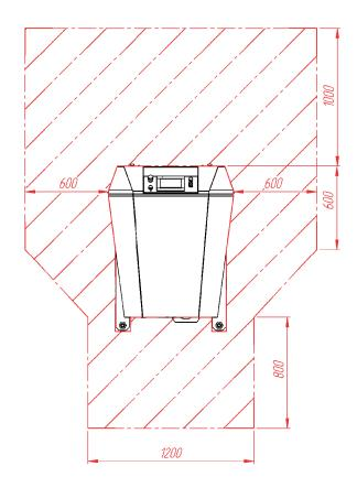
Machine measures and required working space
