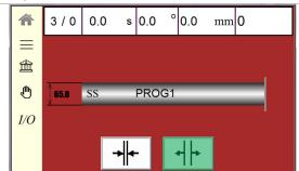
Open the clamps: tap "open clamps" button on the operation panel (lits green), and push one two-hand control button to release tube.
