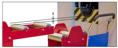
Lift the pipe with a crane to the roller track, use a lifting strap.
