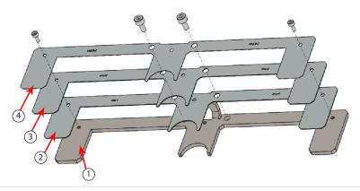
Backstop plates: 1 Base plate, 2. 1st backstop, 3. 2nd backstop, 4. 3 rd backstop
